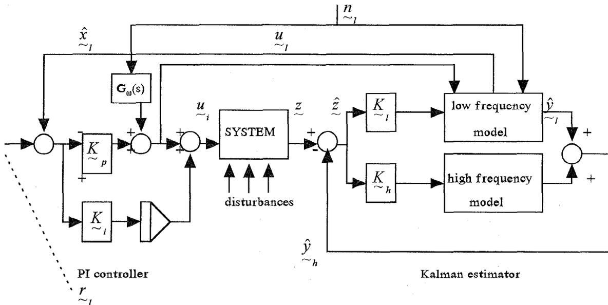
Fig. 2. Dynamic Positioning Control System and Estimator
